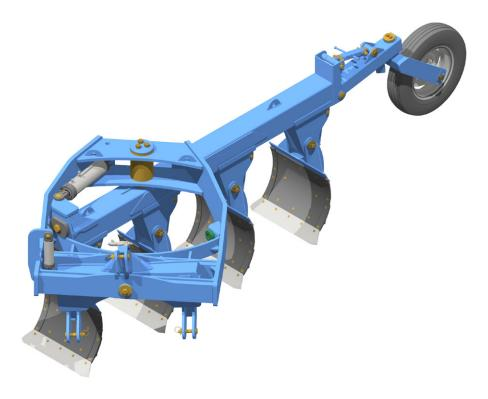
After some hours of operation, the bolts on the plow must be checked to see if they are properly tightened. To assure a great performance and avoid wear and rupture, these bolts must be tightened every so often.
